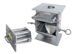
The permanent magnetic separators have been successfully installed throughout companies in the UK, removing fine and weakly magnetic particles from material flow. They are available in 152mm (6") and 203mm (8"), with a stainless steel housing, slide gate to shut off material flow, two banks of Rare Earth permanent magnets to 120°C and suitable for use up to 120°C.
