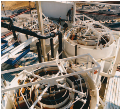
Figure 1. Eriez column flotation cells illustrating froth washing system. Wash water is applied directly into the coal froth to eliminate clays.
