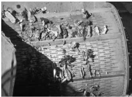
Optional Traction Plate™ improves cleaning yielding a better ferrous product.
