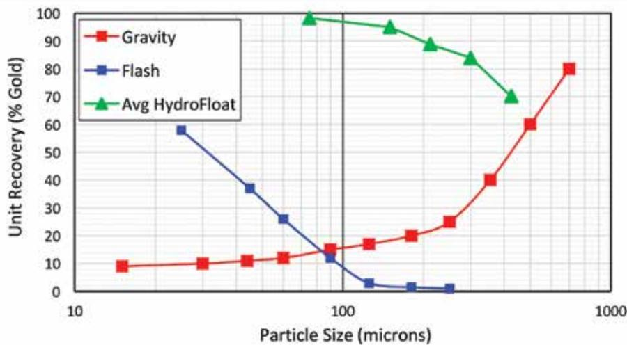
Figure 2: The effective ranges by size for gold recovery, from Seaman and Vollert (2017).
